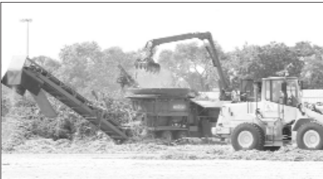
Photo shows tub-grinder at the Northeastern Illinois Public Safety Training Academy in Glenview.
