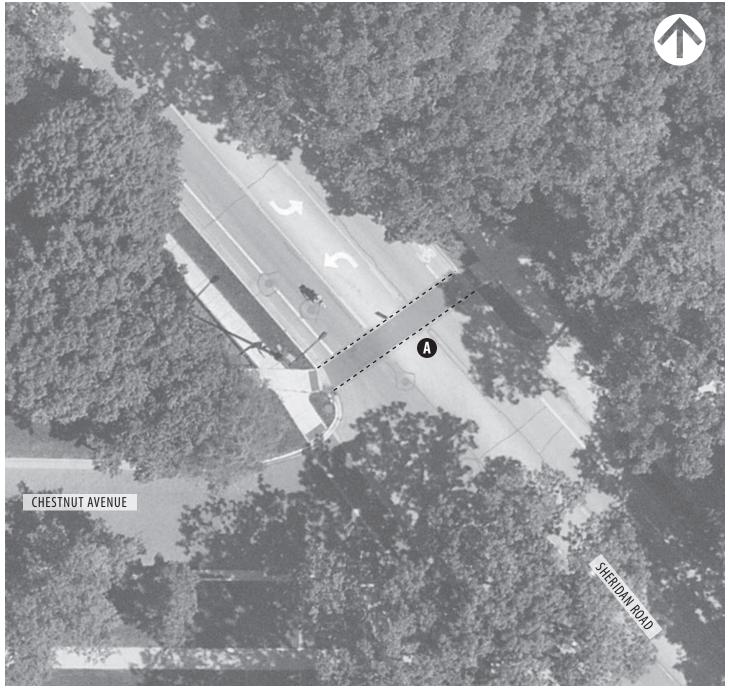
Maintain existing crosswalk and Pedestrian Crosswalk Sign (R1-6a) on-street on the north side of the crosswalk to limit potential impacts by turning vehicles
