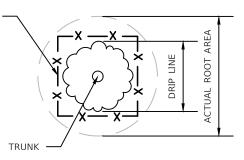
ROOTS OF TREES EXTEND FAR BEYOND THE TREES CANOPY. TO PROTECT THESE ROOTS, PLACE CONSTRUCTION FENCING AROUND THE CRITICAL ROOT ZONE (CRZ = 1' X DBH) OF THE TREE. THE IMPACT OF CONSTRUCTION ON THE TREE WILL LARGELY BE DETERMINED BY THE AMOUNT OF SPACE GIVEN FOR THE TREE PROTECTION AREA.
